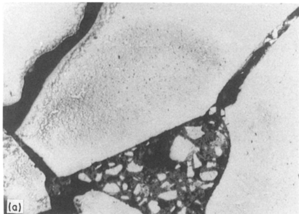
Figure 3 Optical and scanning electron micrographs of SiC-Si 3 N 4 microstructure after oxidation.
